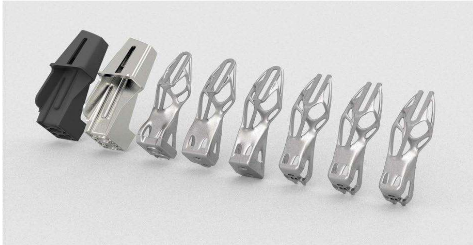
Figure 2 Different results of topology optimization of an automotive manufactured part
