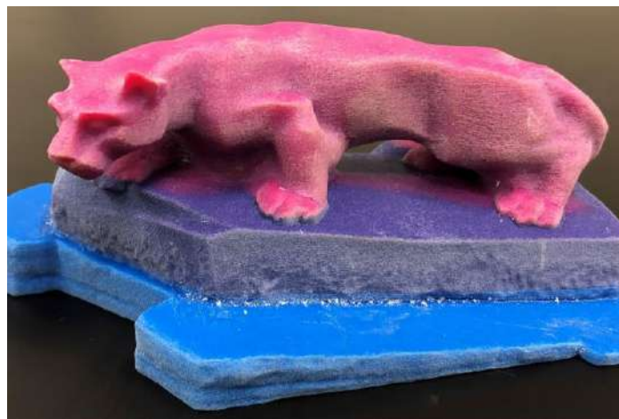
Figure 4. An object produced with Material Jetting technology
