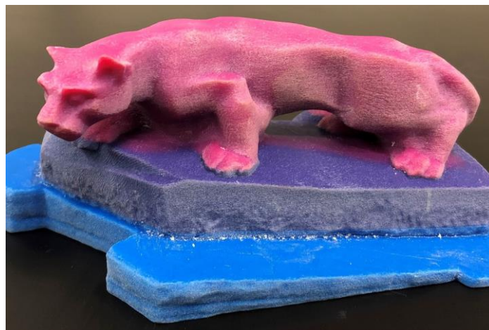
Figure 4. An object produced with Material Jetting technology
