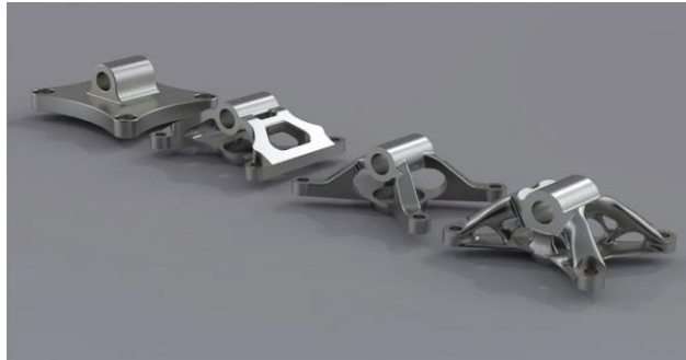
Figure 7. Re-design of components using AM
